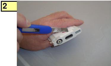
**2** Use a knife to cut the label along the clearance between the cap and the housing
